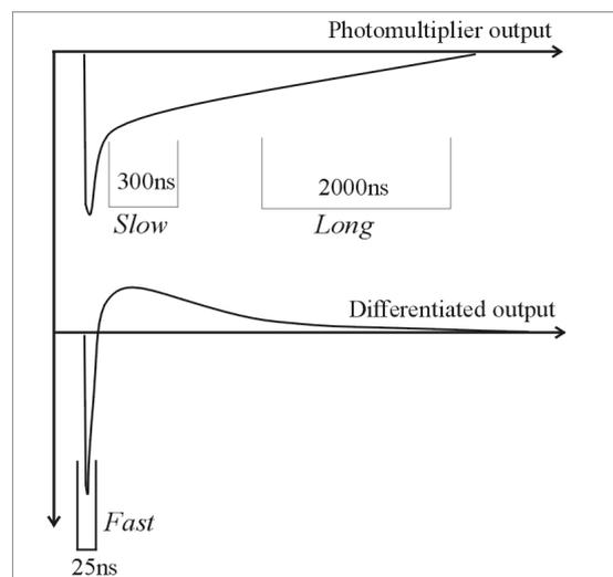
Fig. 7. The phoswich signals with the definition of fast, slow and long gates.
