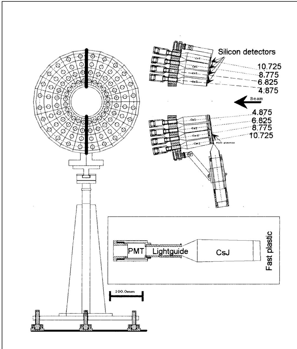
Fig. 1. Forward Wall Detector and Detection Module.
