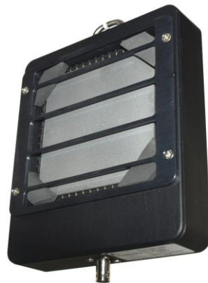
Fig. 2. Beryllium neutron activation detector
