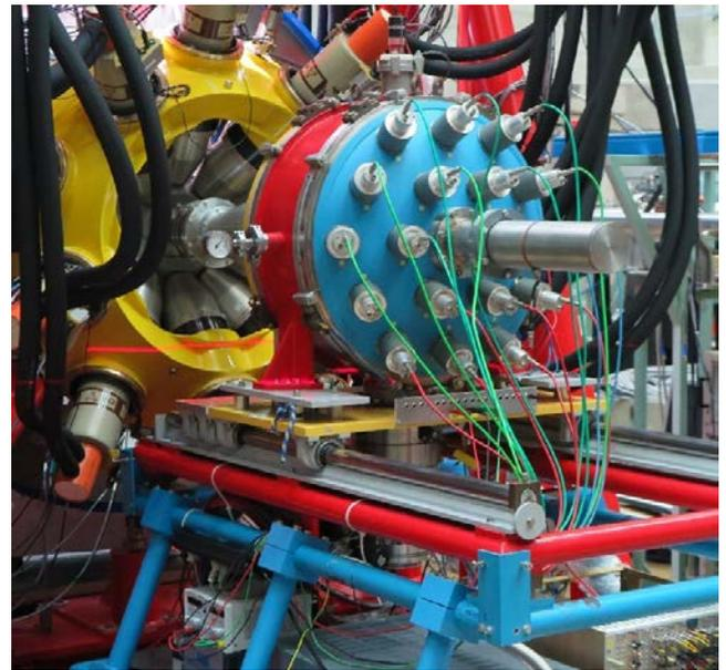
Fig.1 The Recoil Filter Detector coupled with the *GALILEO* array at *LNL*.
