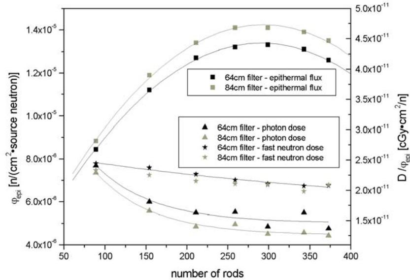
Fig.9. Epithermal neutron flux and the specific photon and fast neutron doses vs. number of rods in 3 cm grid for two widths of the filter/moderator.
