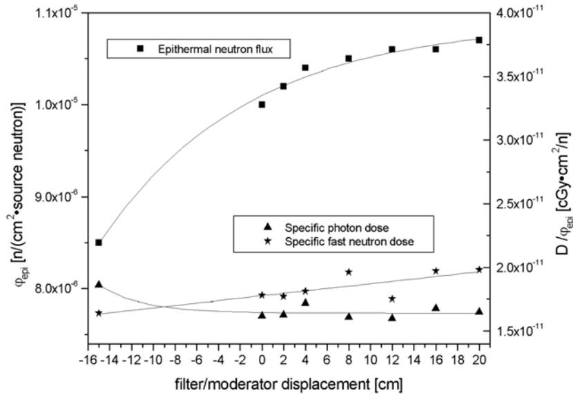
Fig.4. Epithermal neutron flux and the specific photon and fast neutron doses vs. filter/moderator displacement.
