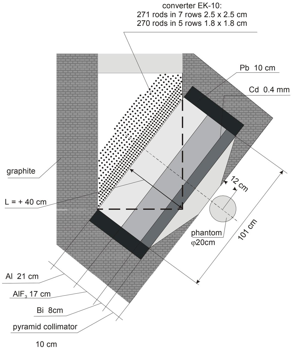
Fig.15. Fission converter with 489 rods arranged in mixed 1.8 and 2.5 cm grid. The filter/moderator width is 101 cm.
