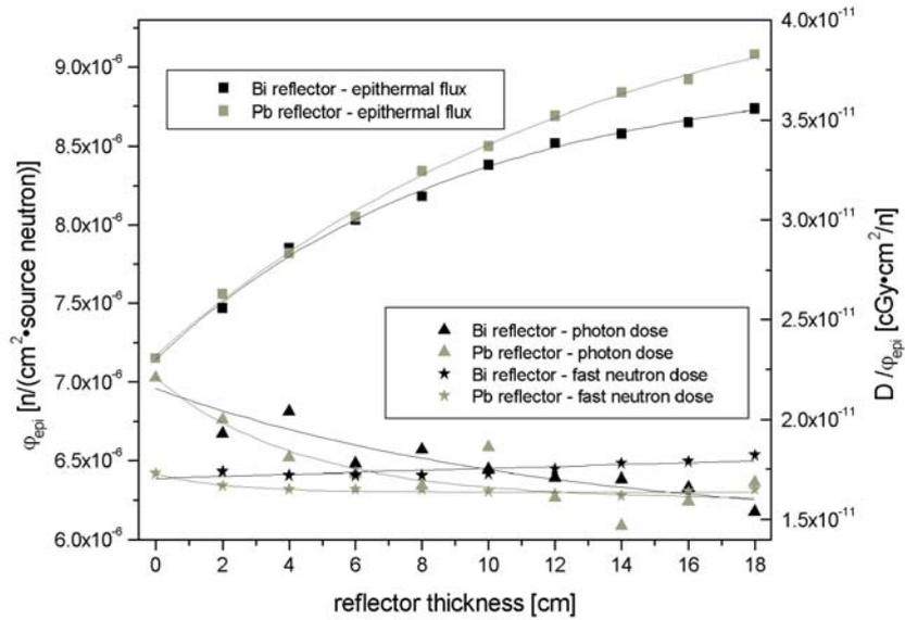
Fig.1. Epithermal neutron flux and the specific photon and fast neutron doses vs. Bi and Pb reflector thickness.
