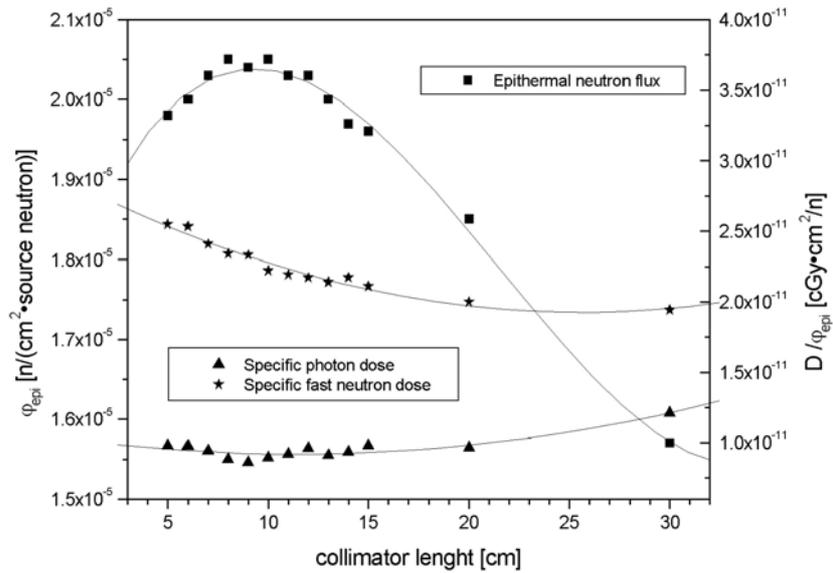
Fig.12. Epithermal neutron flux and the specific photon and fast neutron doses vs. collimator length with no liner.
