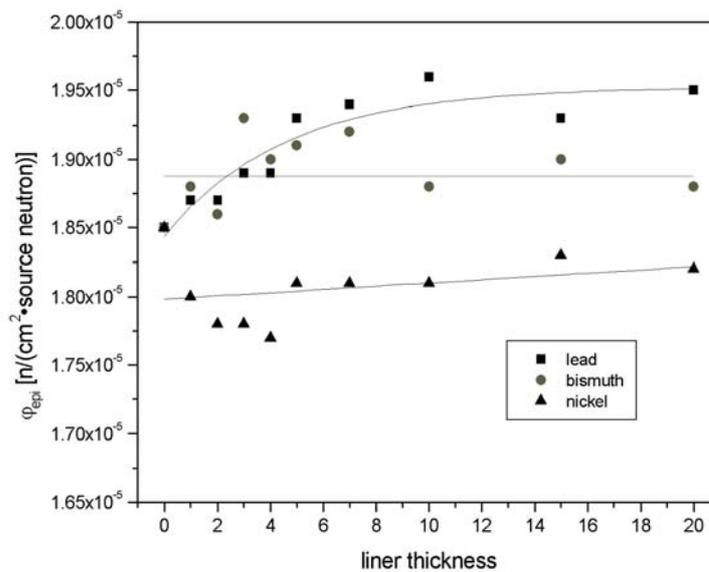
Fig.11. Epithermal neutron flux vs. liner thickness (lead, bismuth and nickel) for 20 cm conical collimator.
