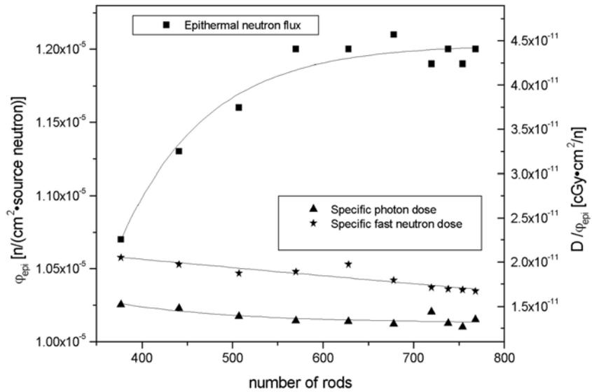
Fig.6. Epithermal neutron flux and the specific photon and fast neutron doses vs. number of rods arranged in two zones.
