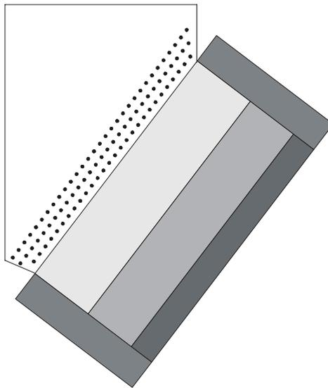
Fig.8. Fission converter with 89 rods arranged in 3 cm grid. The filter/moderator shifted 40 cm toward the reactor duct outlet and widened of 20 cm.
