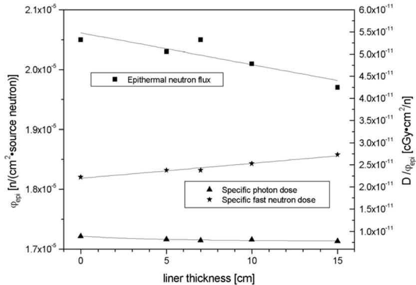
Fig.13. Epithermal neutron flux and the specific photon and fast neutron doses vs. liner thickness for 10 cm conical collimator.
