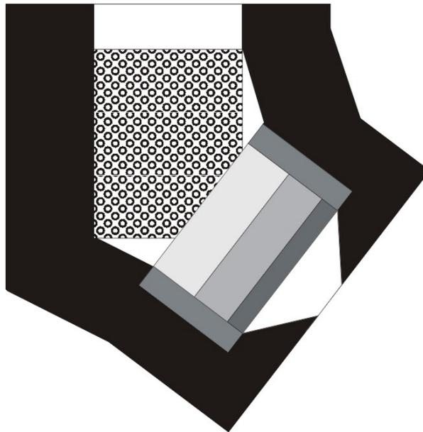
Fig.3. Fission converter and filter/moderator arrangement with the filter shifted of 20 cm toward the reactor duct outlet.
