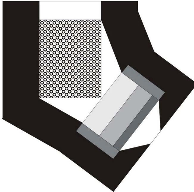
Fig.2. Fission converter and filter/moderator arrangement with the filter shifted as close as possible toward the converter.
