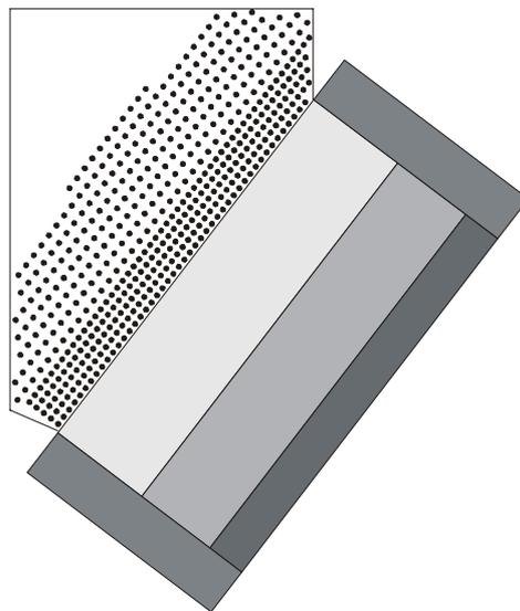
Fig.14. Fission converter with 489 rods arranged in mixed 1.8 and 2.5 cm grid. The filter/moderator width is 84 cm.
