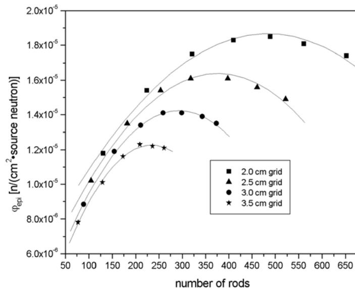
Fig.10. Epithermal neutron flux vs. number of rods arranged in 2, 2.5, 3 and 3.5 cm grids for the filter/moderator width of 84 cm.
