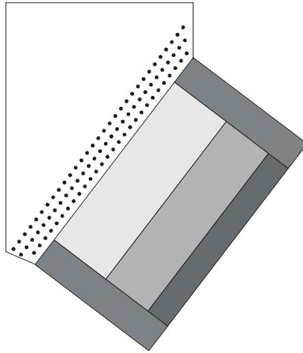
Fig.7. Fission converter with 89 rods arranged in 3 cm grid. The filter/moderator shifted 40 cm toward the reactor duct outlet.
