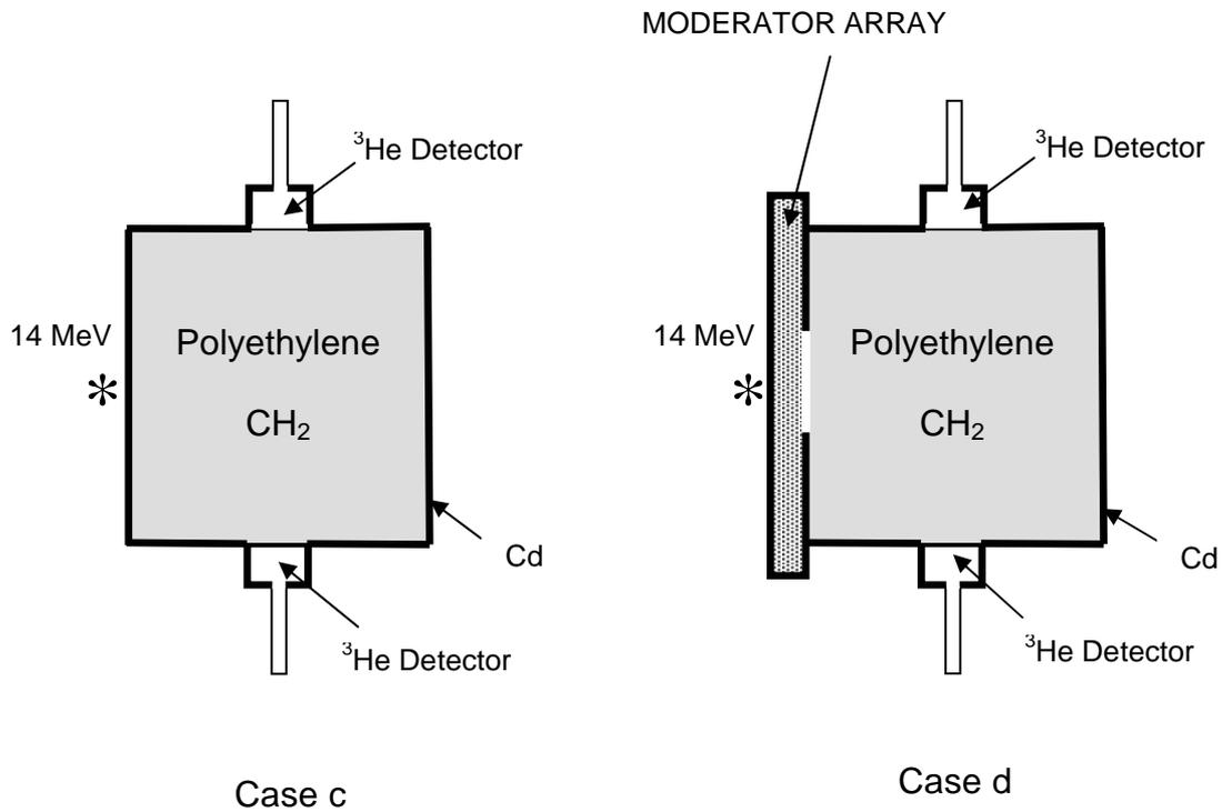
**Fig.4.** Experimental set-up to measure the time decay constant for the sample.
