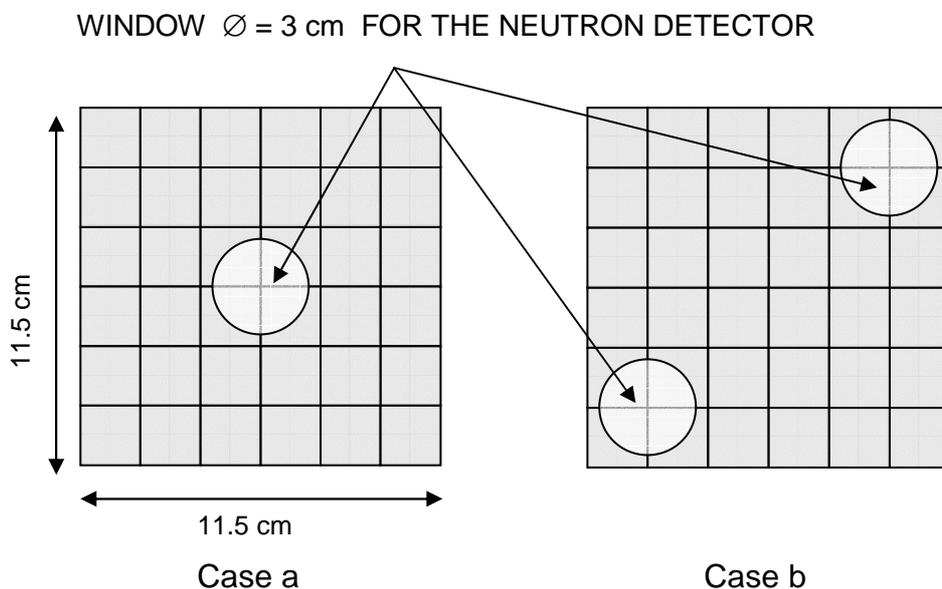
**Fig.2.** Two locations of the detectors at the moderator array.
