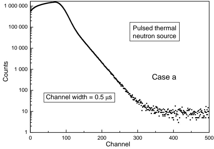
**Fig.3.** Example of the recorded time distribution of the counted pulses.
