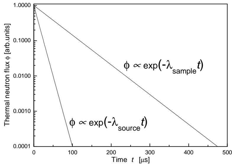
**Fig.5.** Comparison of the thermal neutron decay  $\phi(t)$  in the moderator array and in a sample of polyethylene.
