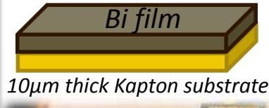
10 $\mu\text{m}$  thick Kapton substrate
