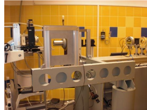
Above - CR plate fixtures in the X-ray positioning system
