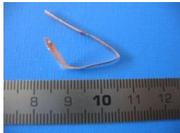
Metallic chip (left) and plastic shaving found and removed during reflectometry and endoscopic (right) inspections of the beam lines
