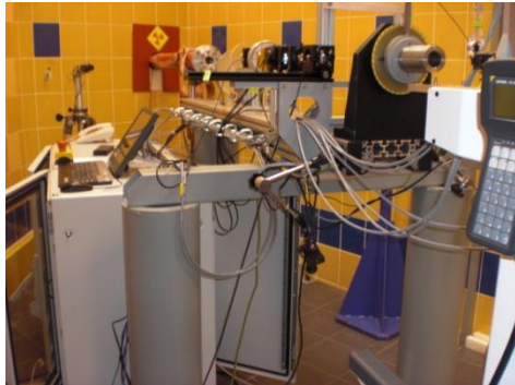
Above - support of the optical bench and its positioning system
