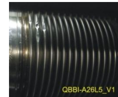
Non-conforming weld (left) and compensation bellow (right)
