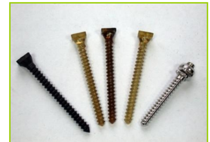
C/C screws as examples of medical application
