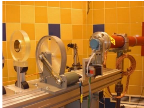
Below - the range-modulating propeller for shaping Spread-out Bragg Peak
